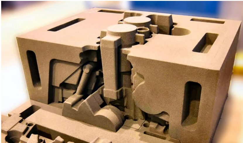
3D printed sand molds and cores can have an accuracy of \pm 0.25\text{mm} and printed in a few days (Source: Castings Technology )
