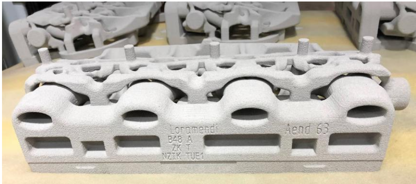
The 3D printed sand core for the cylinder head of the B48 BMW engine (Source: Voxeljet/Loramendi)
