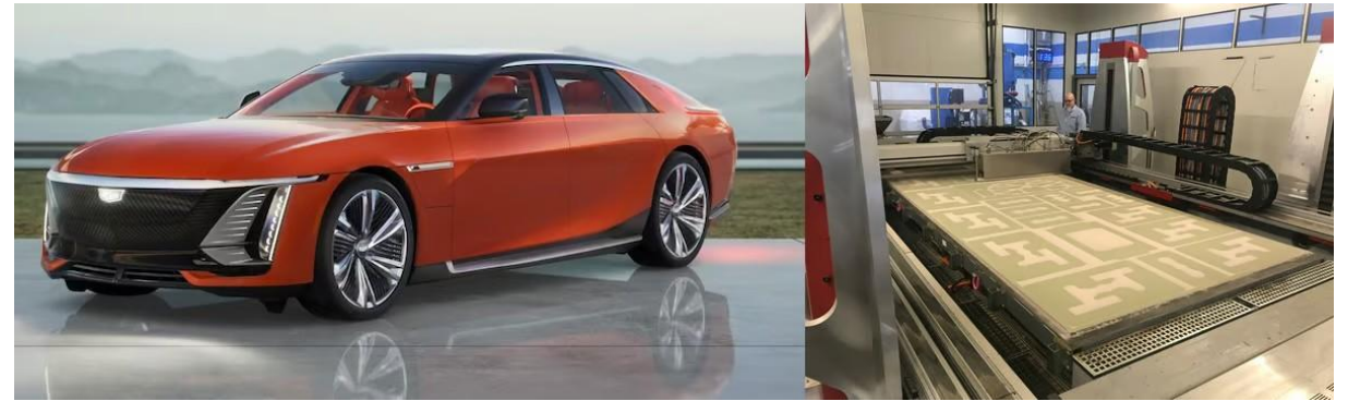
The underbody of the General Motors Cadillac Celestiq is made using 3D printed sand cores that allow for stiffening features to be incorporated into the hollow sections (Source: General Motors, Voxeljet)
