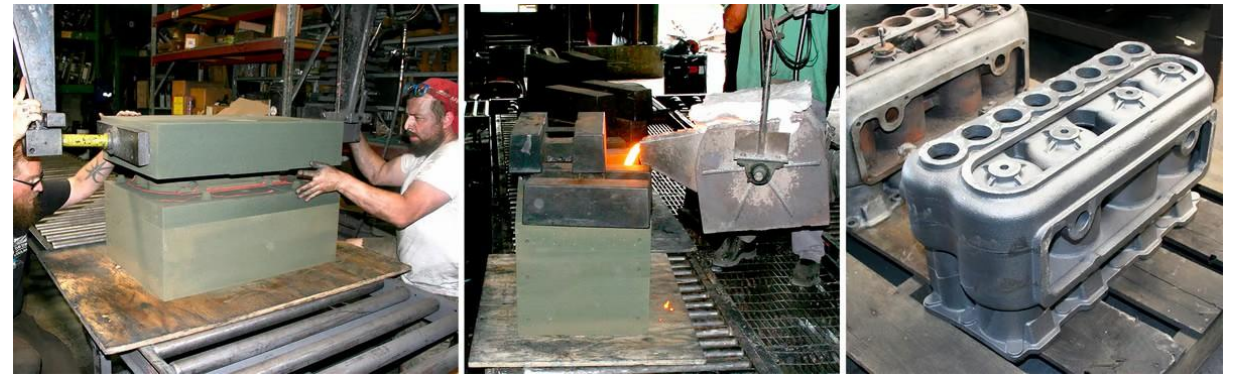
OK Foundry in Virginia uses a 3D printed sand mold to cast a 1912 Velie engine block (Source: OK Foundry)
